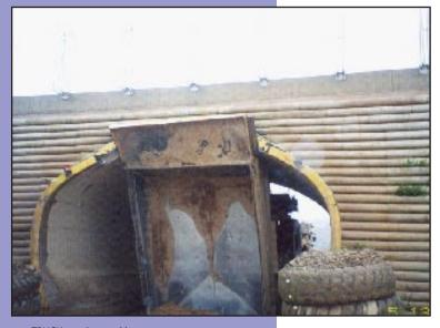
TRUCK tray jammed in underpass, truck wheels off ground
