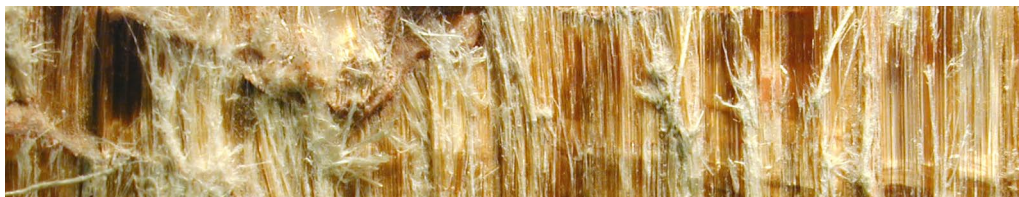
Below: Fibrous Asbestos
